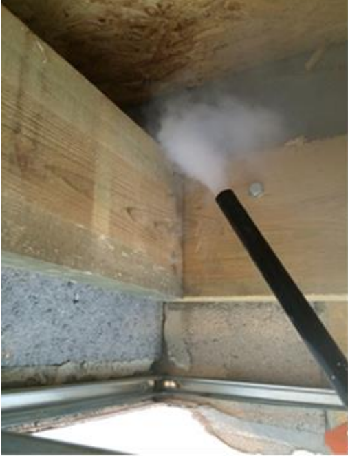
Proving air pathways from contaminated areas
