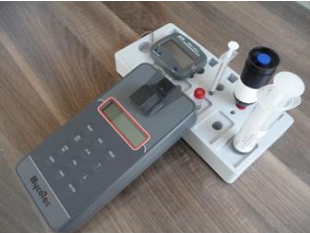
Portable assessments for mould and hyphae presence in air and on surfaces
