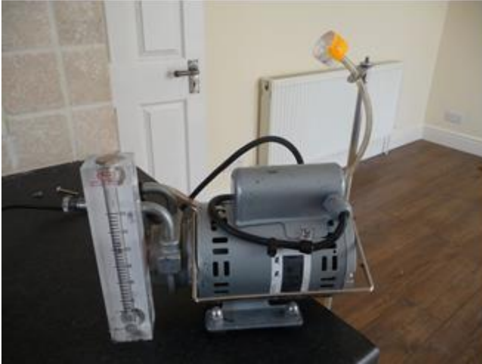
Air pumps used to collect measured samples for lab analysis
